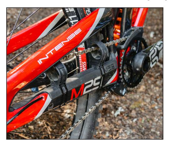
**▼ Gearing:** The STFU chain dampers are designed to work with 1 X setups only. This means if you have more than one front chain ring the system will not function as designed. We have tested using a single larger unit of the TRAIL set with 2X setups (2 front chain rings) and it works on some bikes. At this stage we only offer each system as a set.
